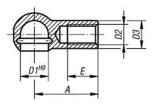
Form B with snap ring and groove for circlip
